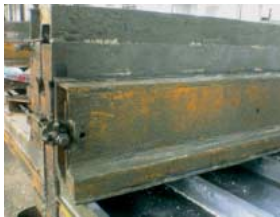
Fig. 1 After work has taken place, the machinery is contaminated with concrete which has partially hardened.
