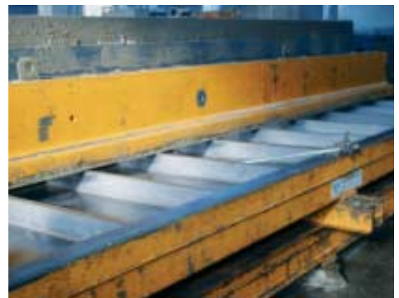
Fig. 2 After treatment of the machine with ZETOLAN MEK, the concrete deposits could be removed without difficulty.
